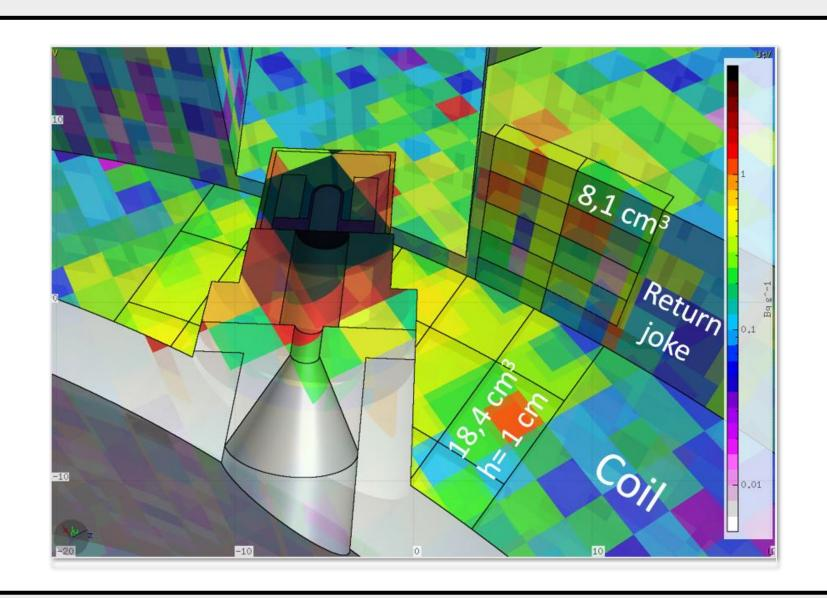
After **two years**, the residual radioactivity is given by  $^{54}$ Mn ( $t_{1/2}$ =312.2 d),  $^{55}$ Fe ( $t_{1/2}$ =2.73 a),  $^{60}$ Co ( $t_{1/2}$ =5.272 a) and  $^{63}$ Ni ( $t_{1/2}$ =100 a). The maximum local activity is from:
