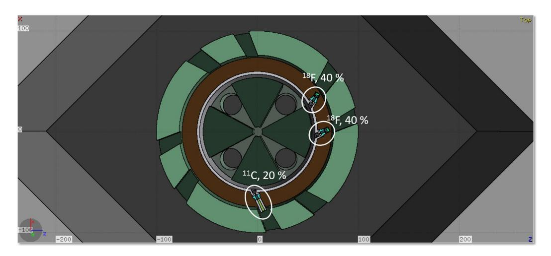
Through FLUKA it was possible to reconstruct the entire working life of the cyclotron: from the operating characteristics (1000  $\mu A\cdot$ week for 20 years), a constant beam has been imposed for 630'720'000 seconds.
