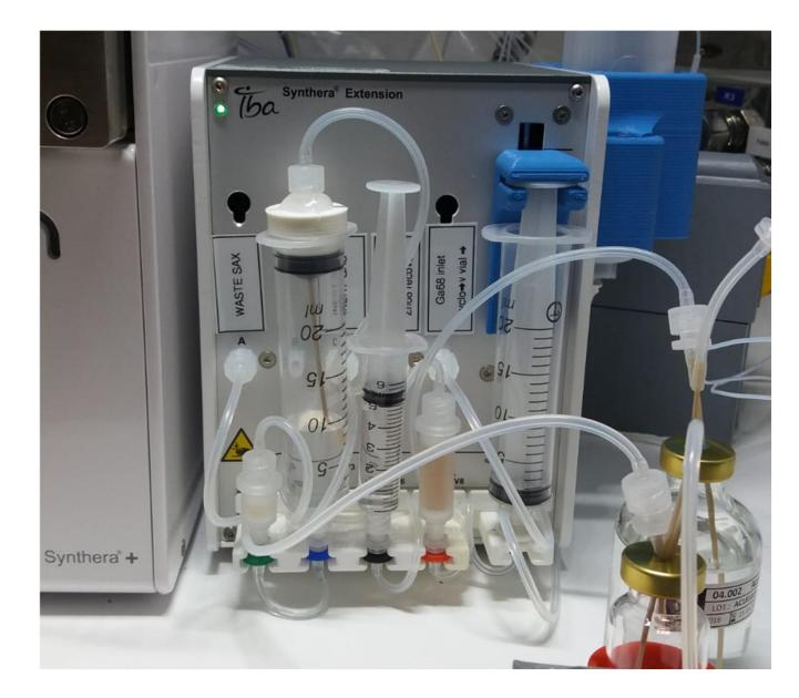
Fig. 4. IBA Synthera®Extension module equipped with Fluidomica purification kit for <sup>68</sup>Ga-target solution
