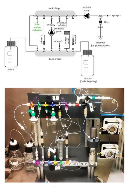
**Figure 6.** Schematic representation of the <sup>44</sup>Sc chemical separation system (above), with the actual system—using disposable medical grade components—shown below. S1, S2, S3 in the scheme indicate the outside syringe lines (containing Bbraun non-return valves) to introduce the solutions used to perform the separation.
