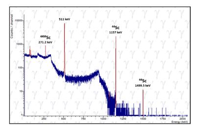
**Figure 7.** Representative  $\gamma$ -spectrum of <sup>44</sup>Sc eluate from irradiated Ca targets, indicating the product is radionuclidically pure.
