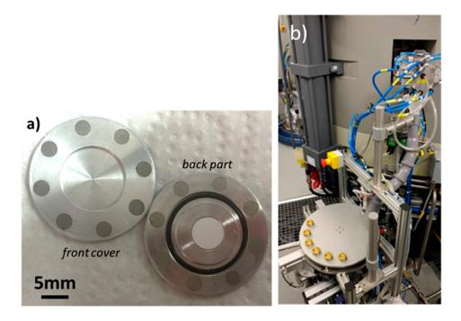
**Figure 4.** (a) Target coin containing a CaO pellet for irradiations using the solid target station at the Bern cyclotron laboratory. The front cover (lid) has a tunable beam entrance window, while the back part (cup) contains the pellet and the O-ring. Once put together, it forms a disc 24 mm in diameter and 2 mm thick. (b) The IBA Nirta solid target station and the solid target transfer system (STTS) installed on the Bern medical cyclotron.
