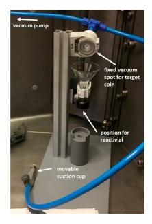
**Figure 3.** Representative picture of the setup used in the hot cell to open the irradiated targets received from the Bern cyclotron laboratory.
