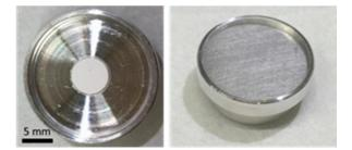
**Figure 2.** Pressed CaO target (6 mm  $\times$  0.5 mm) nestled in the indentation of an Al (99.5% pure) capsule. The capsule was sealed and prepared for irradiation at PSI's IP2 irradiation station.
