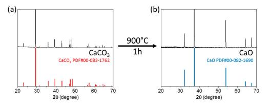
**Figure 1.** X-ray diffraction (intensity) patterns obtained from commercially available  $CaCO_3$  (**a**) and the resultant CaO, obtained after thermal decomposition (**b**).
