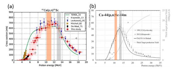
**Figure 5.** Excitation functions of (**a**) <sup>44</sup>Sc (adapted from [21]: reprinted with permission from Elsevier) and (**b**) <sup>44m</sup>Sc (adapted from [26]: reprinted with permission from IOP Publishing) using the <sup>44</sup>Ca(p,n) nuclear reaction. The orange shade (PSI) and gray shade (UniBe) indicates the irradiation energy window of each facility, respectively.
