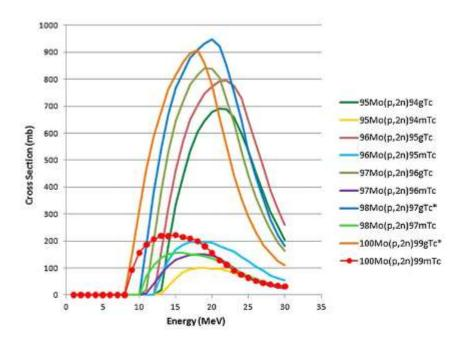
Figure 4. Comparison of the  ${}^{100}Mo(p,2n){}^{99m}Tc$  excitation function to the other radioactive and stable technetium isotopes (isomeric and ground states) which are produced through the (p,2n) reaction. The excitation function for  ${}^{99m}Tc$  is marked with red circles and stable isotopes are marked by an asterisk.
