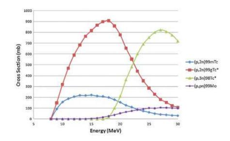
Figure 2. Excitation functions corresponding to the <sup>100</sup>Mo+p reaction products with the highest cross sections in the investigated energy range. Stable isotopes are marked by an asterisk.
