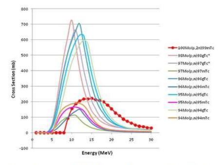
Figure 3. Comparison of the  ${}^{100}Mo(p,2n){}^{99m}Tc$  excitation function to the six other technetium isotopes (isomeric and ground states) which are produced through the (p,n) reaction. The excitation function for  ${}^{99m}Tc$  is marked with red circles and stable isotopes are marked by an asterisk.
