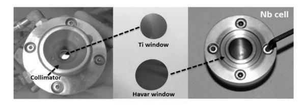
FIGURE 3. *Left*: Target collimator. Centre: Target windows. Right: Target cell
