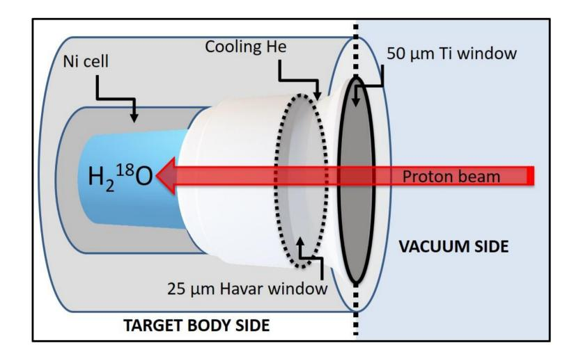
FIGURE 1: structure of the target cell
