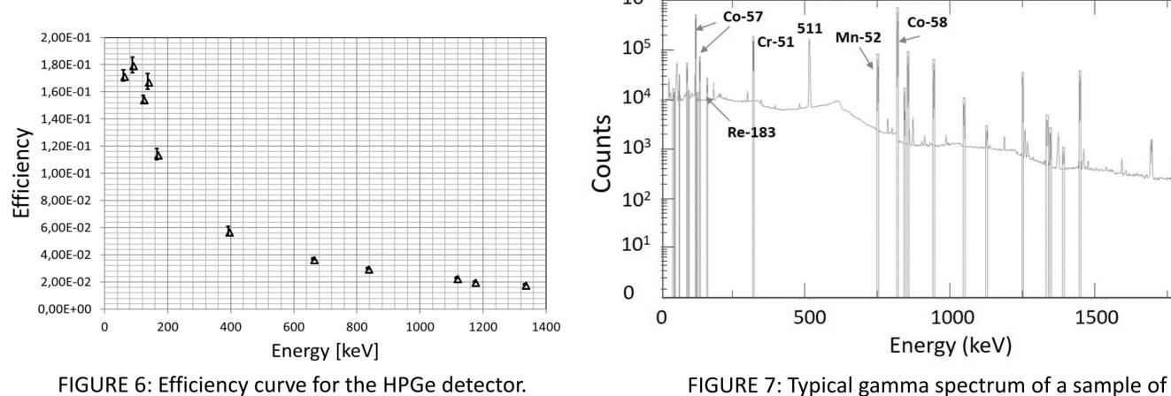
FIGURE 6: Efficiency curve for the HPGe detector.
