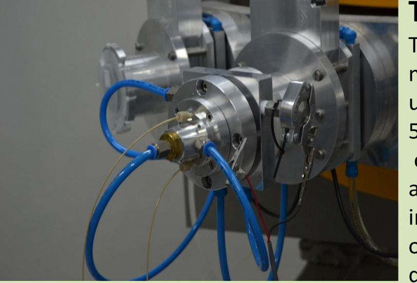
N-13 target being installed in C-30 Cyclotron
