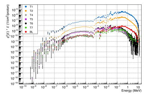
Fig. 8. Neutron fluence at the location of the hotspot of the coils. The contributions from each source are shown separately. The error bars represent the statistical uncertainties of the FLUKA calculations. (For interpretation of the references to color in this figure legend, the reader is referred to the Web version of this article.)
