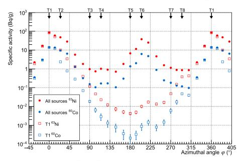
Fig. 9. Azimuthal distribution of the specific activities of <sup>60</sup>Co and <sup>63</sup>Ni for position P1 for a cooling time of 2.5 years. The error bars represent the statistical uncertainties of the ActiWiz calculations. (For interpretation of the references to color in this figure legend, the reader is referred to the Web version of this article.)
