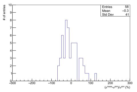
Fig. 12. Distribution of  $(a^{meas} - a^{sim})/a^{sim}$  for <sup>60</sup>Co after normalisation.
