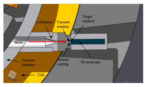
Fig. 3. Target assembly for the production of <sup>11</sup>C. (For interpretation of the references to color in this figure legend, the reader is referred to the Web version of this article.)
