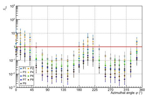
**Fig. 14.** Azimuthal distribution of *S*<sub>LL</sub> after 30 years of cooling. Volumes with *S*<sub>LL</sub> larger than one count as radioactive (points above the red line). Error bars are given at a confidence level of 95%. (For interpretation of the references to color in this figure legend, the reader is referred to the Web version of this article.)
