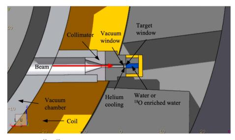
Fig. 2. Target assembly for the production of <sup>18</sup>F or <sup>13</sup>N. (For interpretation of the references to color in this figure legend, the reader is referred to the Web version of this article.)
