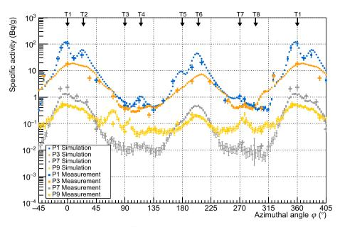
Fig. 11. Simulated azimuthal distribution of the specific activities of <sup>60</sup>Co after normalisation in comparison with measurements. (For interpretation of the references to color in this figure legend, the reader is referred to the Web version of this article.)
