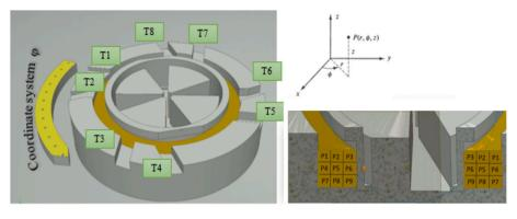
Fig. 4. Schematic view of the cyclotron showing the cylinder coordinates defined for the coils. The positions P1 to P9 are shown on the right. (For interpretation of the references to color in this figure legend, the reader is referred to the Web version of this article.)
