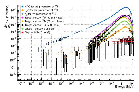
Fig. 7. Neutron energy spectra per primary proton emitted by the different components. The error bars represent the statistical uncertainties of the FLUKA calculations. (For interpretation of the references to color in this figure legend, the reader is referred to the Web version of this article.)
