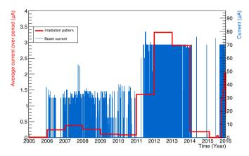
**Fig. 5.** Blue curve: beam current as a function of time. Red curve: average beam current per time interval (period). The period was set to one year for the years 2004–2014 and to one month for the year 2015. (For interpretation of the references to color in this figure legend, the reader is referred to the Web version of this article.)
