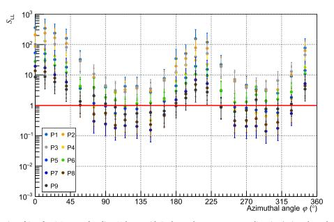
Fig. 13. Azimuthal distribution of  $S_{LL}$  after 2.5 years of cooling. Volumes with  $S_{LL}$  larger than one count as radioactive (points above the red line). Error bars are given at a confidence level of 95%. (For interpretation of the references to color in this figure legend, the reader is referred to the Web version of this article.)
