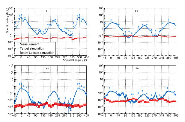
**Fig. 10.** Azimuthal distribution of the specific activities of <sup>60</sup>Co for the positions P1, P3, P7, and P9. Simulation results are compared to measurements. The contributions from targets and beam losses are plotted separately for the simulation. (For interpretation of the references to color in this figure legend, the reader is referred to the Web version of this article.)
